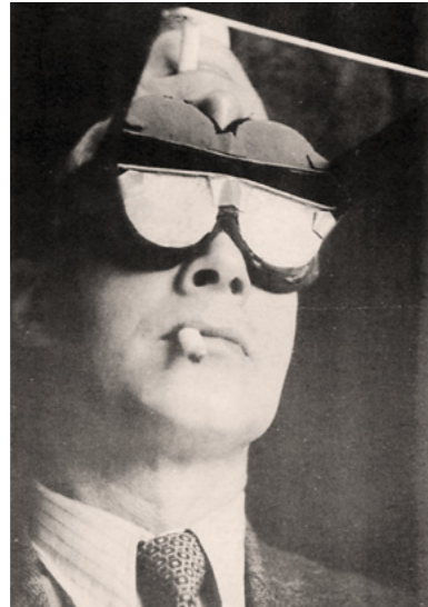
Prism glasses as used by Erismann. A specula turns the image upside down. The field of vision is 80 degrees vertical and 40 degrees horizontal.
